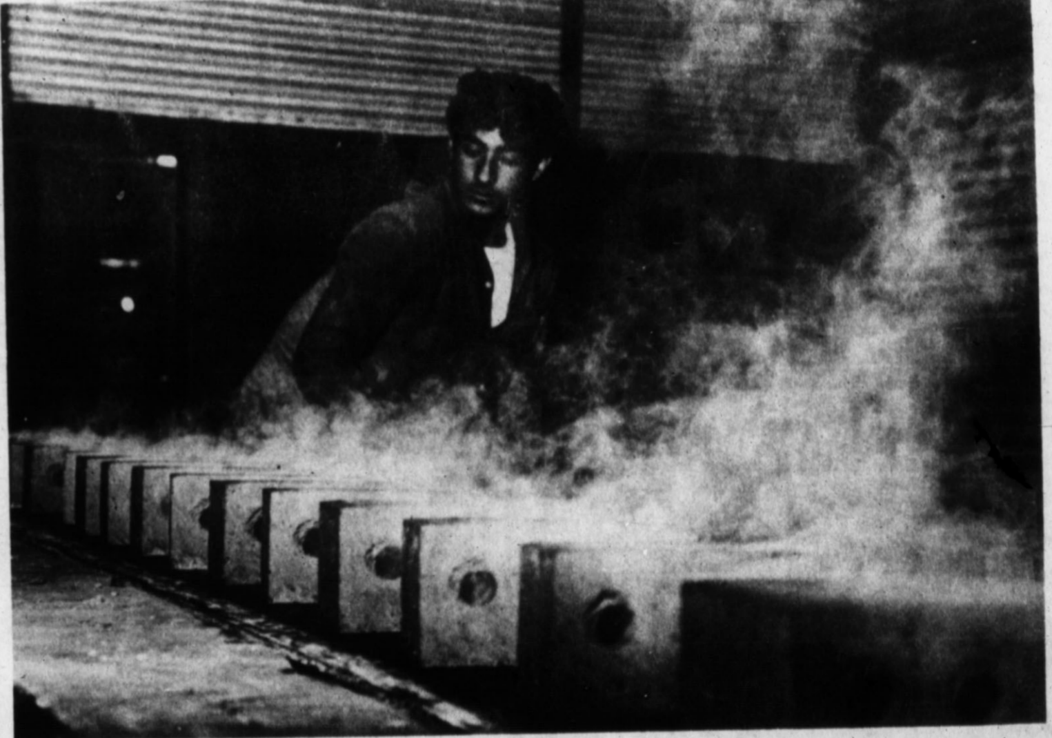
A STEAMING COLUMN OF BRICKS parades along the conveyor belt at Hereford Tile and Brick Company's local manufacturing plant. Waiting to stack the brick on carts is Tony Vallejo. The brick have been freshly cut and are still warm from being heated. They will next be placed in dryers for three days and then into kiln for nine more days, where they will be heated to some two thousand degrees Fahrenheit. The local manufacturing plant will reach peak production within two weeks after recent modernization and addition of new machinery. (Staff Photo)
