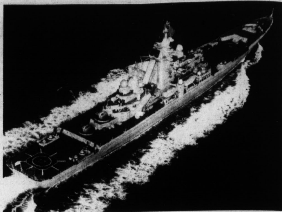
THIS SOVIET BATTLE CRUISER is the biggest warship apart from aircraft carriers to be built by any country in more than 30 years. The 32,000-ton "Kirov," shown here running trials in the Baltic Sea, is equipped with SA-N6 and SA-N3 missiles and with 30 millimeter guns for rapid fire. The ship is more than 810 feet in length and more than 88 feet in the beam.
