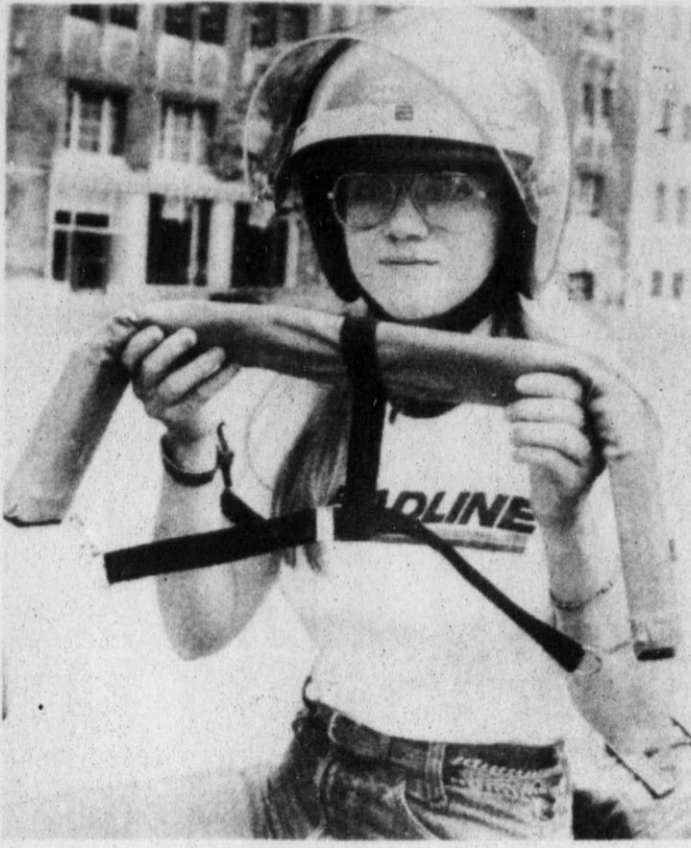
THE LATEST IN radios is this AM-FM stereo model that transmits sound through the bones when worn as a scarf. The new radio is said to be considerably safer than headphones for people like motorcycle messenger Eva Mrgan because it does not muffle extraneous noises such as horns and sirens.
