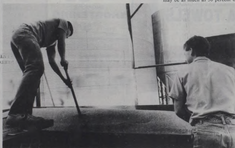
RYAN KLEMENT probes a load of wheat at Muenster Milling for a moisture test before unloading the grain brought in by Ashley Fuhrmann of Lindsay. Janie Hartman Photo
