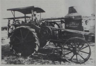
THE MODEL H,16-30 Advance Rumely Oil Pull Tractor appeared in 1919. The two-cylinder engine operated at 530 rpm and developed a 4,674-pound drawbar pull and cranked out 32.52 brake horsepower. Production ended in 1924, with a total of 56,647 oil pulls being built in 14 different models.
