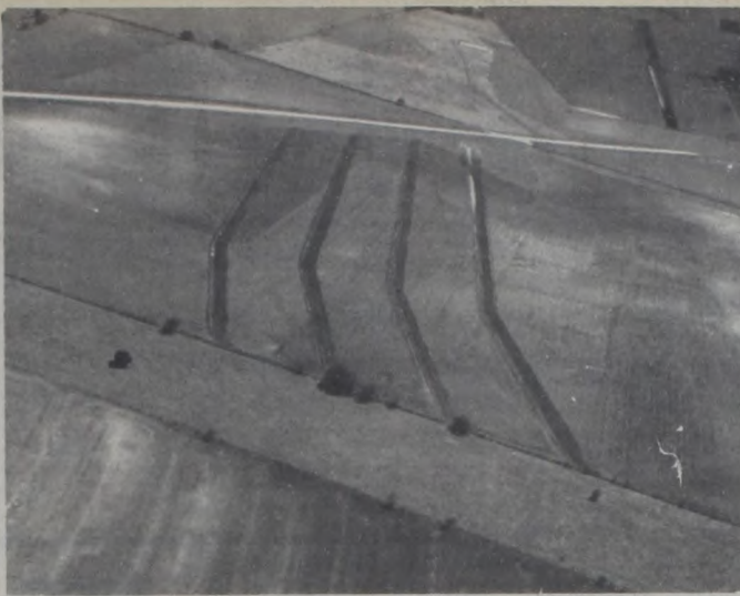
Here you see the end result of a topographic map which included four terraces and waterway which has been recently installed.
