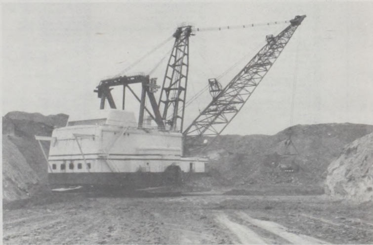
Mike Murphy, TP&L Manager, Gainesville gives an idea of the immense size of dragline scoop used in the strip mining operation. This 70 cubic yard scoop is awaiting repair.
