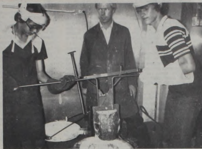
Just before pouring a cast, students Bryan Hoenig and Donnie Lutkenhaus lift a crucible of molten aluminum from an electric furnace. Rudy Koesler, instructor, is in the background supervising.
