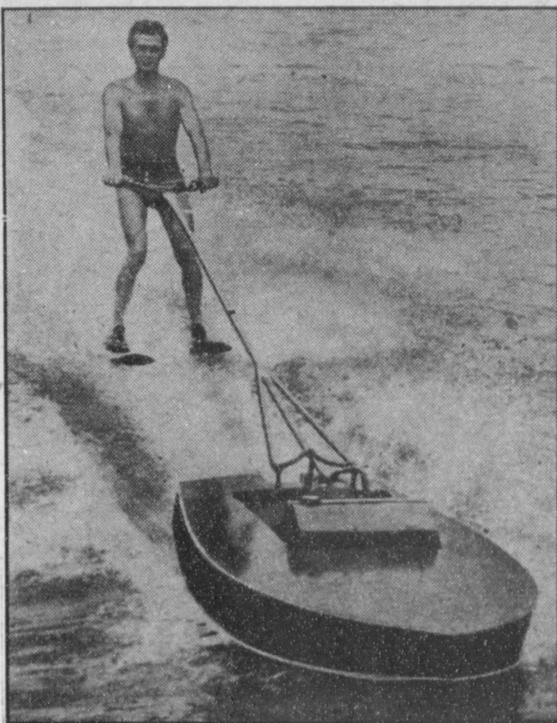
ONE-MAN SKI RIG —To go bounding over the billowy main on water skis it usually takes quite a crew. This new invention, demonstrated at Klagenfurt, Austria, would simplify all that. The six-foot motor tug has a 10-foot steering and control mechanism. The model will do 25 miles per hour, and the inventor hopes to have the speed up to 50 miles per hour when he markets the gadget.
