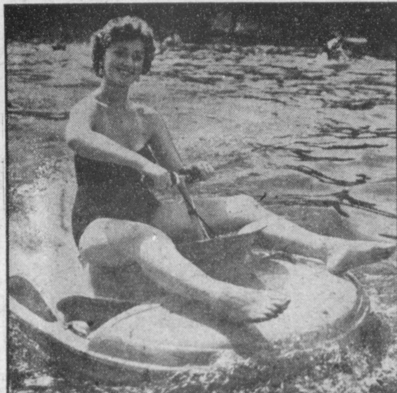
MARINE SAUCER —Tiny, gasoline-motor-driven water scooter makes its debut in West Berlin, Germany. It put-puts over the waves at about 10 m.p.h. and is steered with a motor scooter-type handlebar.
