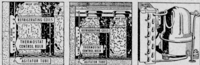
NEW ice bank control: Action No. 1. Adjustment is provided to control ice bank to suit altitude, climate, load.
