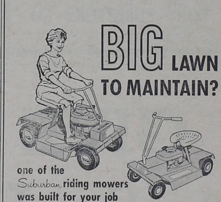
There are two: the big Suburban 26, with its 26-inch cut, 41/2-hp engine (automatic impulse starter) and a dozen fine-mower features. And there's the Suburban 24, that cuts a full 24-inch swath, has a rugged 31/2-hp engine, plus many features of the Suburban 26, including forward and reverse speeds up to 3.6 mph, one-pedal control, and safety blade lockout.
