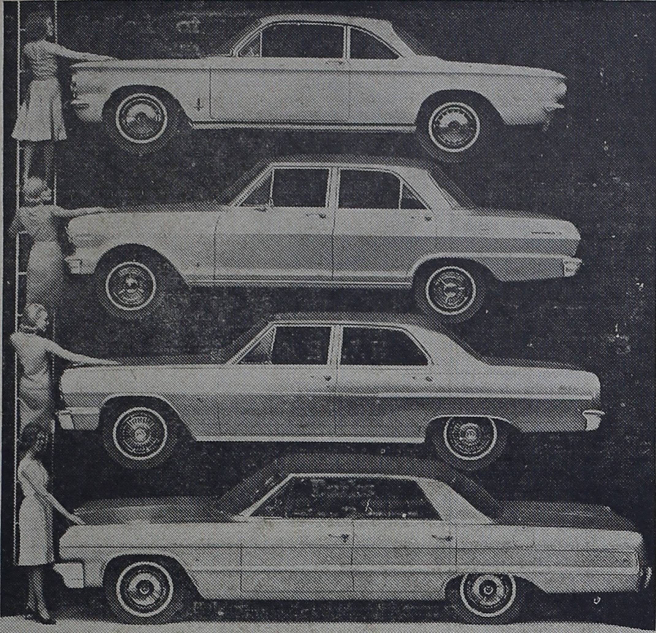
For 1964, the Chevrolet Motor Division will offer a total of 43 models in five separate passenger car lines. Each line is distinguishable by its own styling and wheelbase. Above, reading down: the 108-inch wheelbase Corvair Monza Coupe; 110-inch wheelbase Chevy II Nova 4-Door Sedan; the newest car in the Chevrolet family—the Chevelle Malibu 4-Door Sedan which has a wheelbase of 115 inches while the Chevrolet Impala Sport Sedan is built on a 119-inch wheelbase. Not shown is the Corvette Sting Ray which sports a 98-inch wheelbase. Chevrolet dealerships will have a representative showing of all models when the new cars are introduced September 26.
