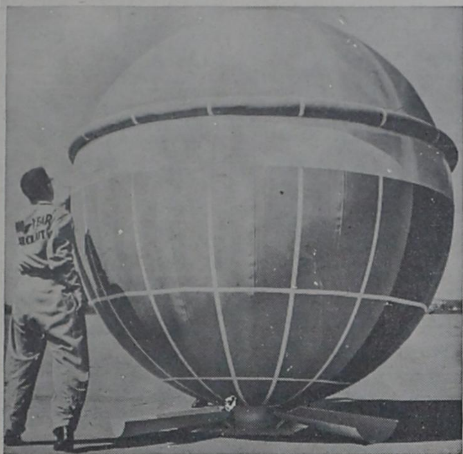
ROUND FIGURE —This ballute—balloon plus parachute—is capable of inflating in one tenth of a second to control the high-speed deceleration of manned and unmanned re-entry vehicles. The 9-foot diameter balloon eases the vehicle through the critical heat barrier of the earth's atmosphere.
