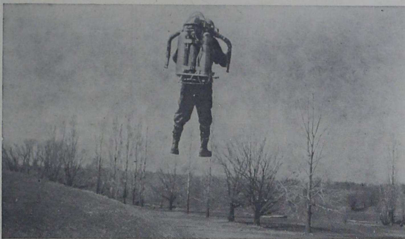
NO VISIBLE MEANS OF SUPPORT — Bell Laboratories engineer Harold Graham becomes the first man to fly a back-pack rocket. He rose 30 feet into the air in Buffalo, N.Y., and wooshed over the ground for about the distance of a football field.
