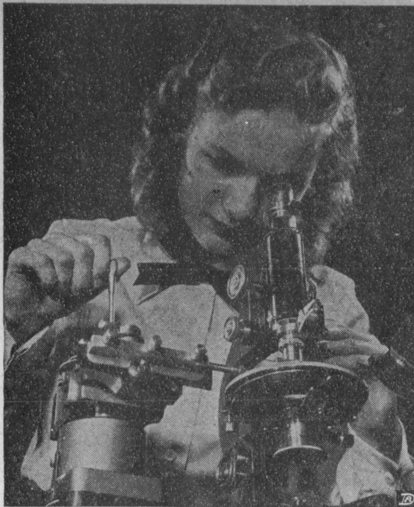
HARMARVILLE, PA. —Particles invisible to the naked eye are handled by this wizard-like machine of modern science, called the micro-manipulator. The hand lever operates a hydromatic drive directing probes, rakes and shovels so tiny they work within a drop of water as would ordinary instruments in a beaker or test tube. A humidified cell prevents evaporation of the minute sample beneath the microscope lens. Photo was taken at Gulf Oil's micro-laboratory where research into the infinitely small is speeding progress toward meeting the world's demands for oil.
