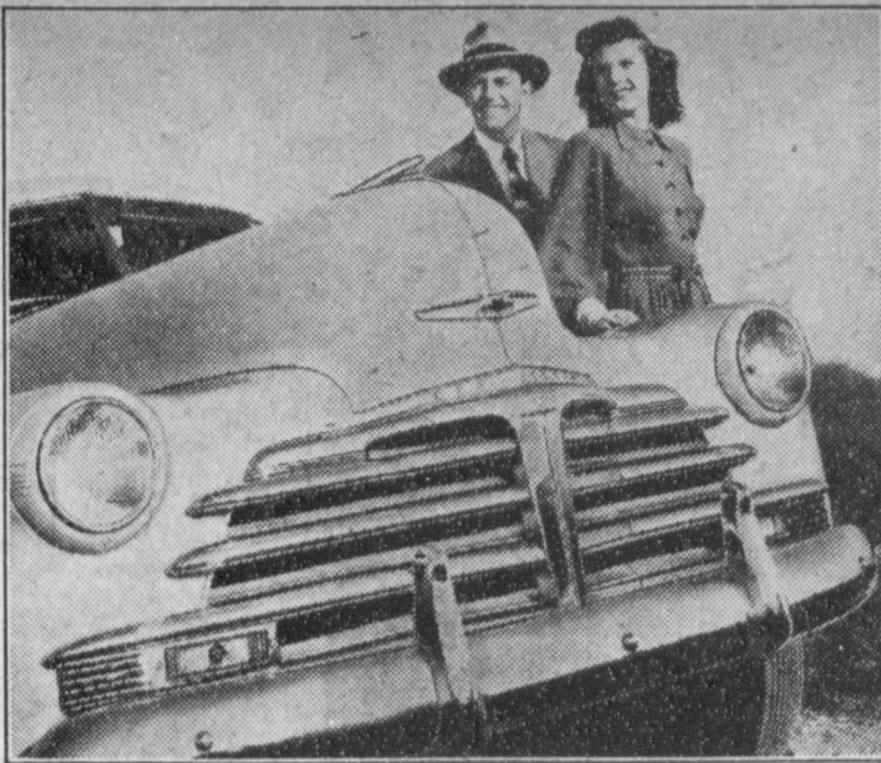
The front of the new, 1948 Chevrolet, showing the redesigned radiator grille, has been changed by the addition of a modernistic, T-shaped chrome center bar. The smooth contours of the front end, with fenders and hood blending in form, are shown here.
