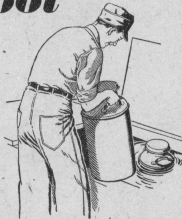
This type of cooling tank, with cool water circulating around milk cans, is a practical, effective arrangement.
