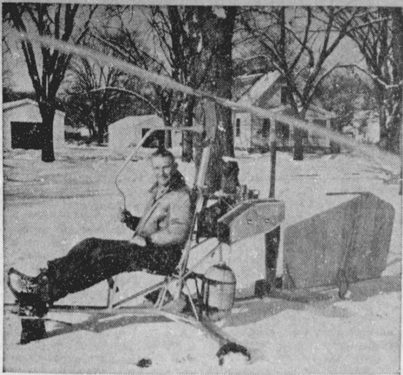
IT FLIES? —That's what it's designed to do. Al Wilson, of Topeka, Kan., constructed this machine from various oddments, including a 72 h.p. engine. The machine weighs but 225 pounds.
