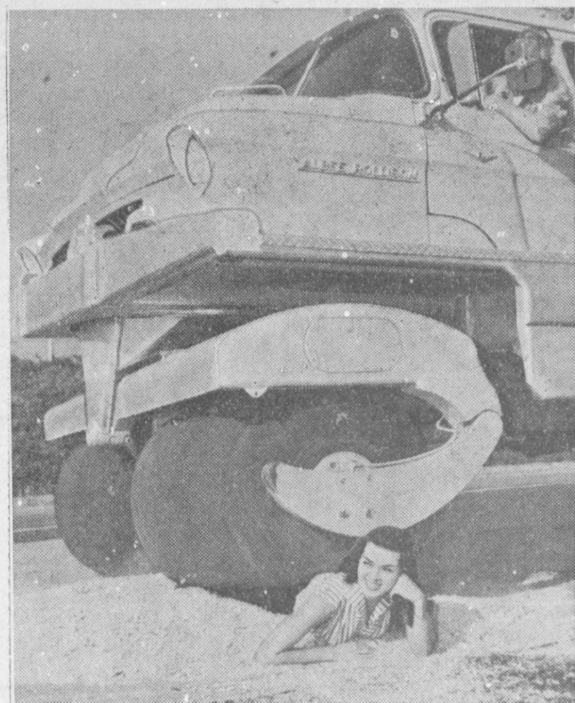
FEELING NO PAIN — Smiling Cindy O'Hara, 18, "Miss International Auto Show," bears up very well under the strain as seven tons of truck rolls over her in San Francisco. The unusual vehicle, which moves on huge, sausage-shaped pneumatic pillows instead of conventional wheels and tires, is called the Rolligon. On display at the 32nd annual San Francisco International Auto Show, the truck is able to "absorb" rocks and other obstacles (like Cindy) by "flowing around them." It is able to carry heavy loads over very rough ground.
