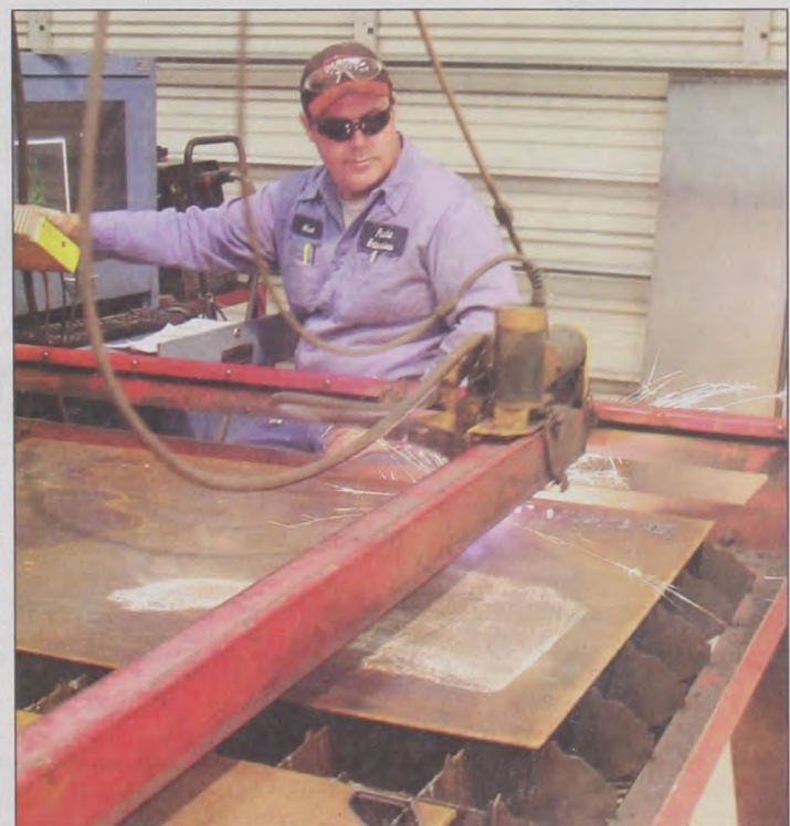
Neal Flusche operates CNC plasma cutter at Flusche Enterprises, Inc. to custom design a sign. Janie Hartman photo
