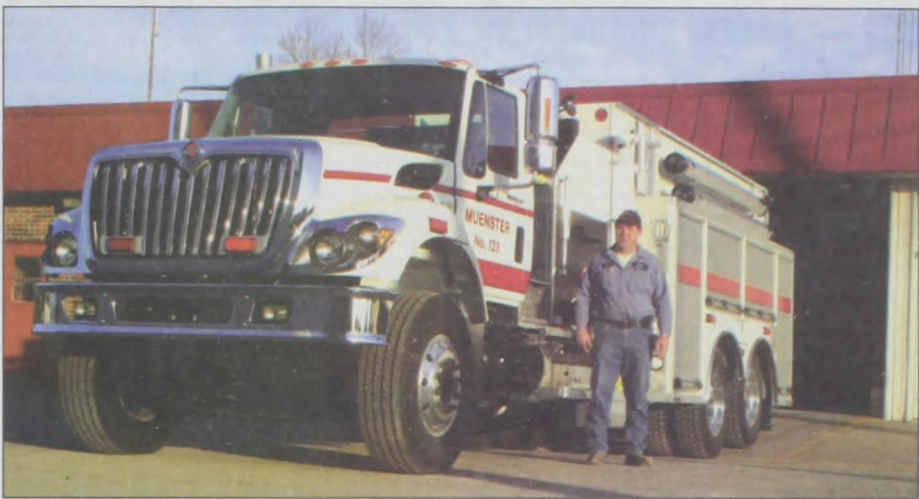
Muenster Volunteer Fire Department members were excited this week to finally see their new fire truck in Muenster. They purchased a 7500, SBA, 6x4, International Truck last summer and sent it to Waco to have a 2500 gallon tank with a 1250 gallon per minute pump built onto it. The finished truck is now being equipped with hoses and other necessities. It should be ready for use in a few weeks. Fireman Neal Flusche is pictured. He is a member of the MVFD Fire Truck Committee. Janie Hartman photo
