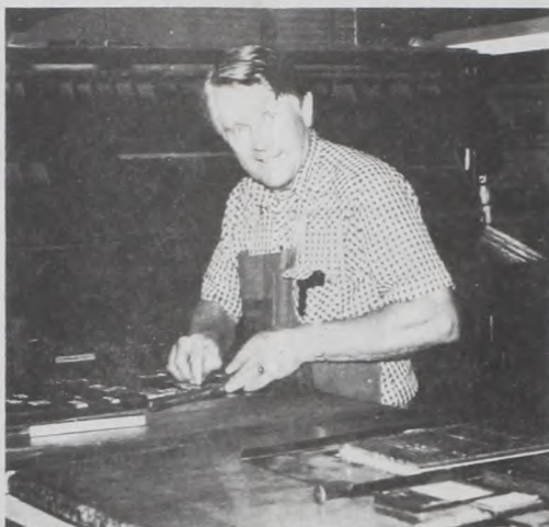
Alvin Hartman completes the last page using hot metal type to be printed by the letter press method, before the Muenster Enterprise converted to offset in 1980. He celebrated his 50th anniversary of employment with the Enterprise in September. Janie Hartman photo
