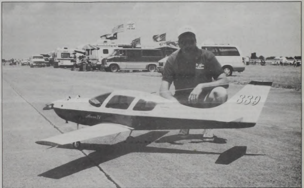
BILL CUNNINGHAM of Tulsa, Oklahoma is the winner of the unlimited class race in the Lone Star Unlimited Aviation Expo held at Gainesville Municipal Airport last week. He won all his heats and the trophy race with this scale model Lanceair IV. The aircraft is powered by an 8.8-cubic-inch engine which develops 25 horsepower and is capable of 200 miles per hour in level flight. Cunningham, who has been flying model planes for 24
