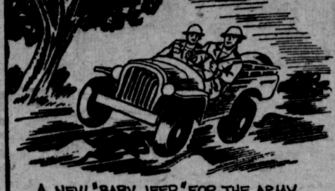
A NEW "BABY JEEP" FOR THE ARMY WEIGHS ONLY A THOUSAND POUNDS, CARRIES TWO PEOPLE AT 50 M.P.H. AND CAN POSSIBLY BE DROPPED BY PARACHUTE.
