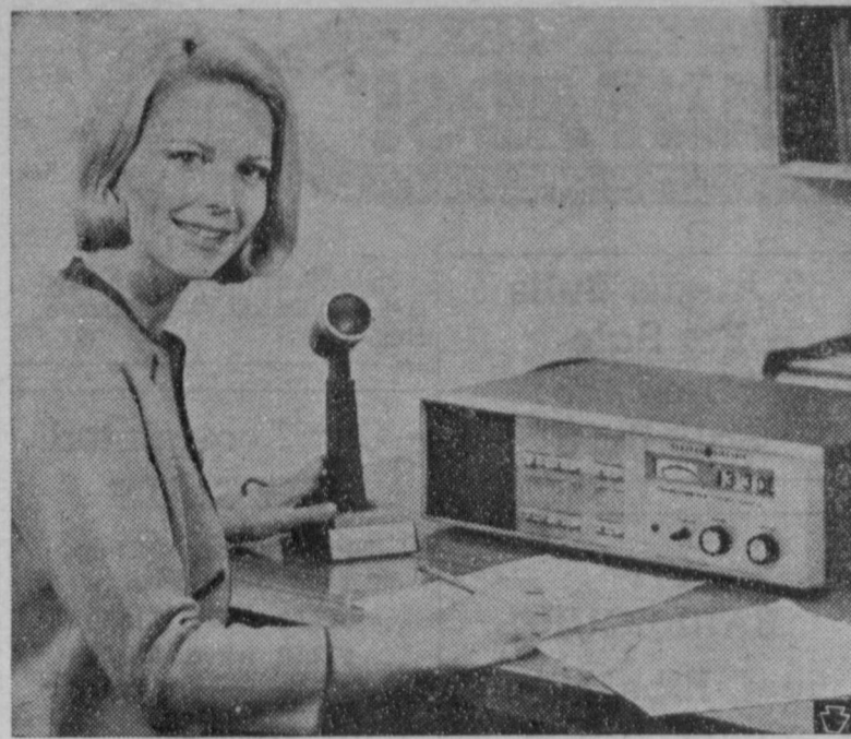
New remote control console for FM two-way radio system compensates electronically for changes in outgoing voice levels of different dispatchers, and provides anti-blast protection for incoming calls. Designed by General Electric at Lynchburg, Va., for use by businesses, governmental agencies and others, it's all-transistorized, easier to operate and more functional. Another automatic feature, electronic voltage regulation, keeps the console's performance steady and provides extremely stable characteristics for messages to cars and trucks on the road. For multi-office locations, additional consoles may be used.
