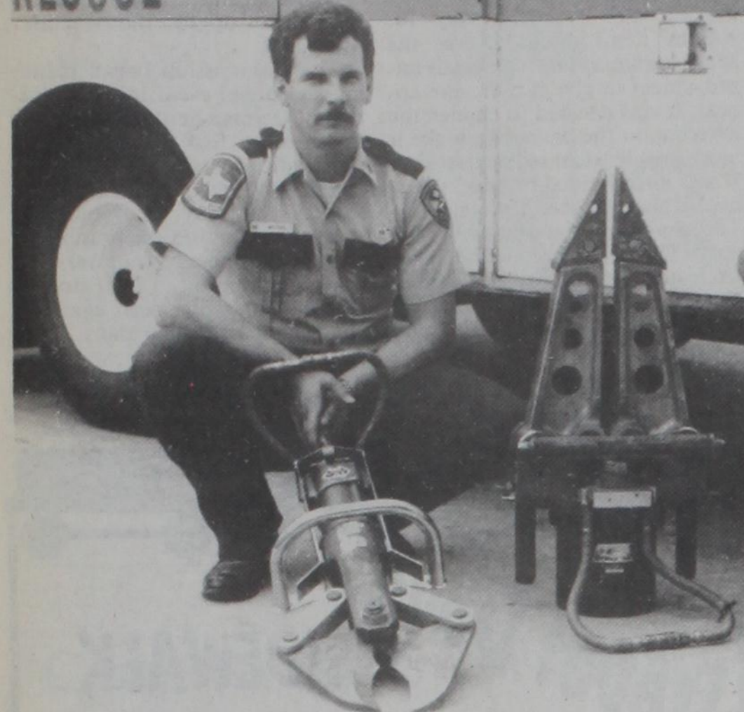
CAPT. WES REED displays some of Cooke County EMS's rescue equipment. Best known as the "Jaws of Life," the tools are used to pry open vehicles when trapped victims are in need of immediate medical attention. The cutters can free someone in 30 seconds when other methods could take 10-15 minutes. Janie Hartman Photo
