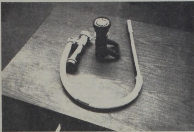
Shown above is the new foam inductor recently acquired by the Volunteer Fire Department which will be used as an aid in fighting oil and gas fires in the future.
