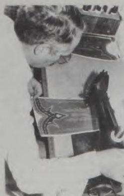
CUSTOM bootmaker sews a fancy stitch design on boot tops using a 1930 commercial sewing machine.
