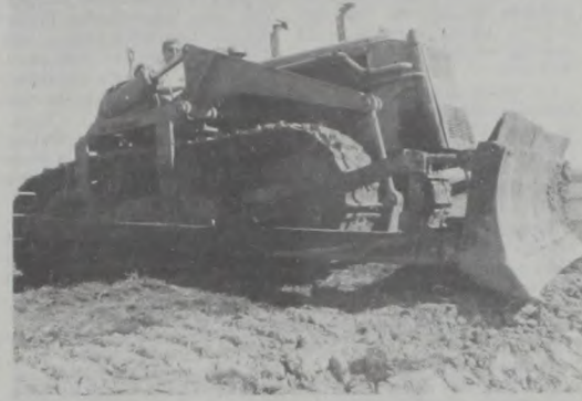
WEIGHING about 36,000 pounds, this used International bulldozer has been purchased to perform compaction and dirt work at the landfill.
