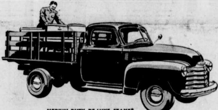
MEDIUM-DUTY DE LUXE STAKE* Model 3609—125½-inch wheelbase, Maximum G.V.W. 5,800 lb. Other models available up to 161-inch wheelbase and 16,000 lb. G.V.W.
