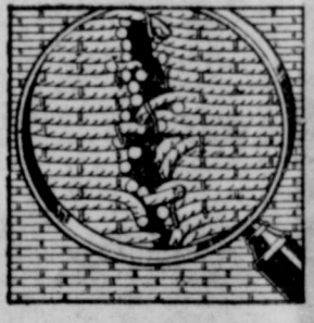
Cord Separation This shows how cords inside tires other than Riversides are separated by heat. Cord separation causes internal blisters, weakens the tire. A blowout is the result! Riversides are Blowout Proof because of Latex dipping!
