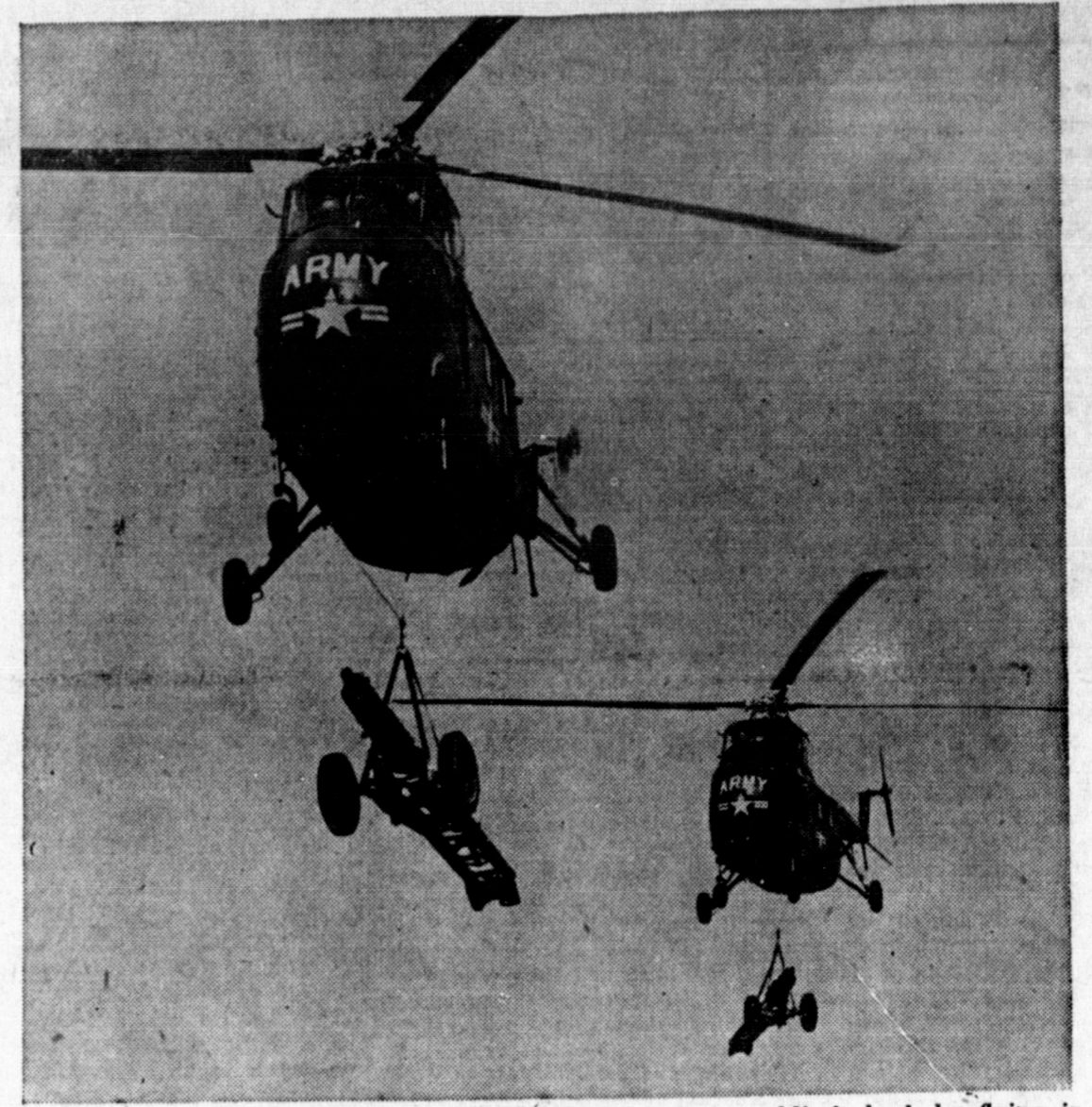
Army H19 Sikorsky helicopters take the burden off the soldier's back by flying in 75mm pack howitzers during training maneuvers at the Army Aviation Center, Camp Rucker, Ala. This helicopter is used also to carry soldiers into simulated battle areas.
