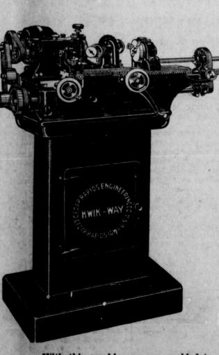
With this machine we are enabled to **Reface Rocker Arms Reface Valves Grind** Commutators **Do Lathe Work True Tappets Repair Expansion**, Spiral and Straight Reamers **General Auto Repair Work** FINIS HARP'S AUTO HOSPITAL
