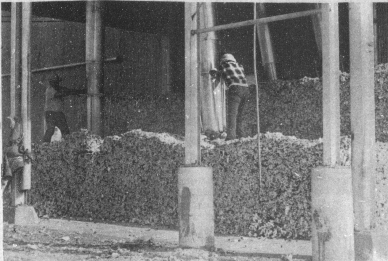
GINS OPERATING AT FULL SPEED --Taking advantage of good weather, cotton gins throughout the area are operating at full speed. This scene, at Muleshoe Co-op Gin, is a familiar sight at any cotton gin operating in the area at this time. Here, the two suction operators are sending a module through the gin.
