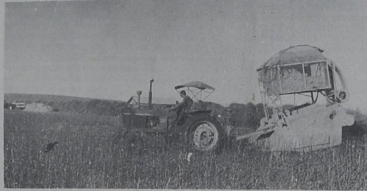
BUTCH COLLINS uses a Rood to clean fields of cotton left by ordinary cotton picking machines.
