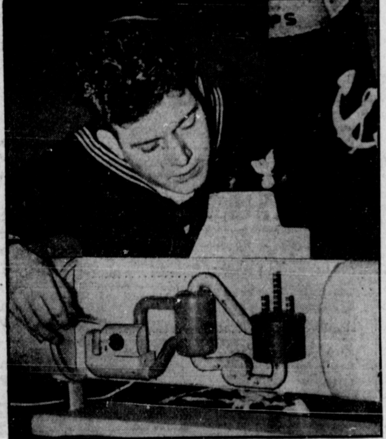
ATOMIC TUMMY—Checking the atomic-engine-filled stomach of this model of the submarine Nautilus, on exhibition at Atlantic City, N. J., is Electrician 1/c. William Christian. The vessel, now under construction at Groton, Conn., will be the world's first atom-powered sub. It will be capable of running for months under water at a speed of 20 knots.
