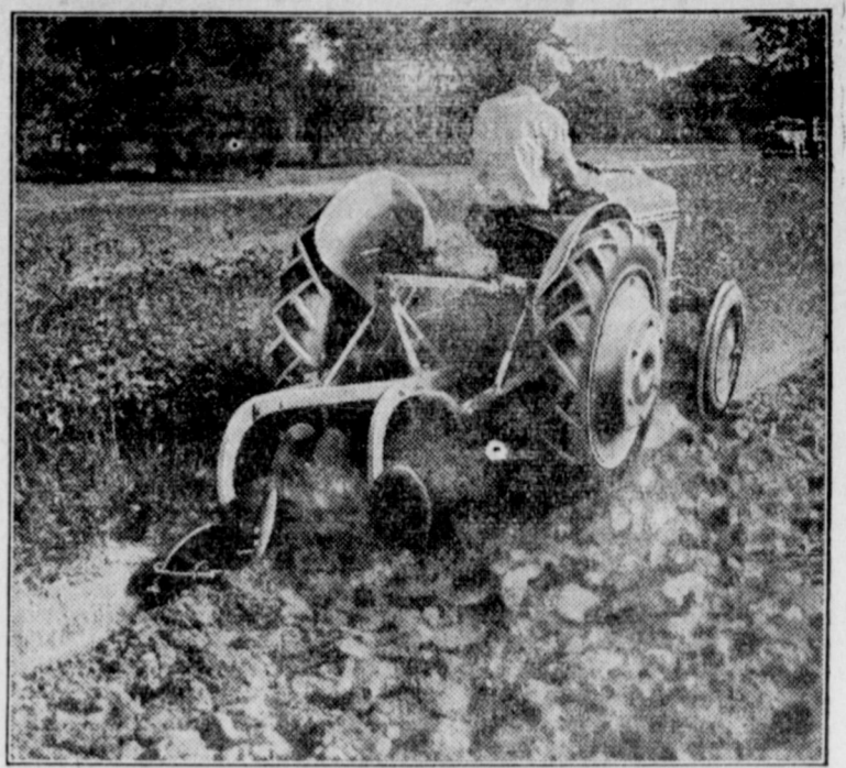
PHOTO SHOWS the new Ford tractor with Ferguson plow in action. The operator merely steers in a straight line to obtain perfect plowing results. The Ferguson system hydraulic mechanism keeps the plows at a uniform depth and operates without attention except at the ends of the field. Then a convenient, easily-operated lever is moved to lift and lower the plow when turning. The tractor pulls a two-bottom 14-inch plow with ease, and because of its light weight gives remarkably low fuel consumption, average fuel consumption being one gallon an hour. The tractor with plow attached can be turned on an eight-foot headland, and worked in fence corners.
