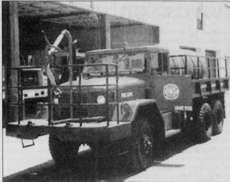
Fox 1 The Clarendon Volunteer Fire Department put a new grass fire truck into service last month. The six-wheel drive unit, dubbed "Fox 1," replaces an older truck and has the capacity to carry 1,000 gallons of water. Generous donations of time, skills, supplies, and resources from local businesses and citizens helped bring the truck online.
