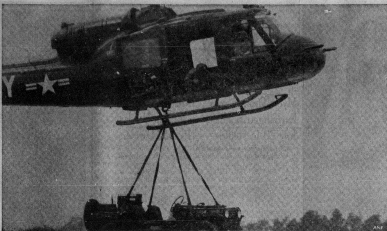
SHOCK TREATMENT — Jeep-mounted radio equipment gets the "once over" from an airborne rigging specialist during the air transportability phase of a service test conducted at Fort Bragg, N.C., by the Airborne, Electronics and Special Warfare Board. The board is an activity of the U.S. Army Test and has Evaluation Command. Purpose of the test is to determine what effects air transport has on radio equipment.
