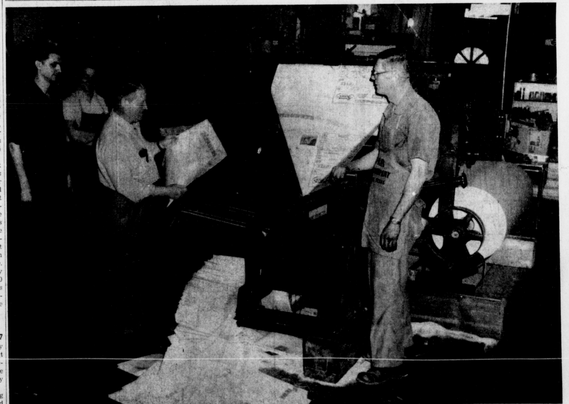
This is how the Goss Comet roll-fed press appeared Tuesday when a trial run was being made. Pressman John Just is shown at right pushing the lever to put the press in operation which is quite a contrast to the other press operation where each sheet had to be hand fed, printing 4 pages and then flopped over and 4 pages printed on the other side. Checking the press over, left to right, Bill Tipton, Ernest Moreland, and Editor Estlack.
