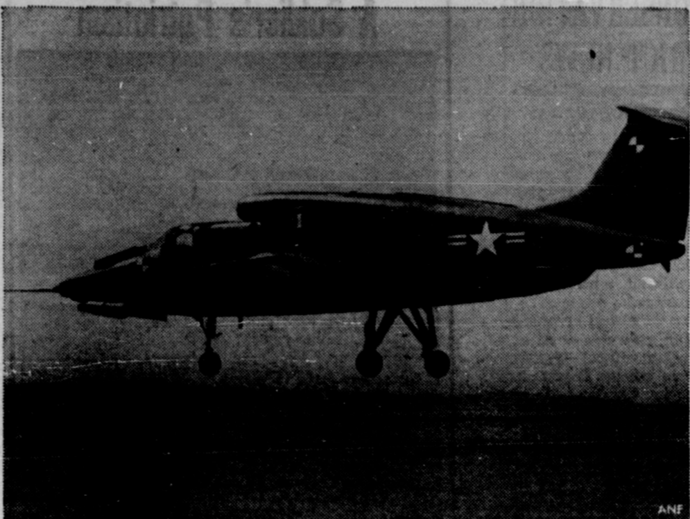
SUCCESSFUL HOVER—The U.S. Army's experimental aircraft, the XV-5A, demonstrates hover flight at Edwards Air Force Base, California. The fixed wing aircraft rose vertically on the jet thrust provided by two wing fans and a nose fan, hovered motionless, and then descended slowly for a landing.
