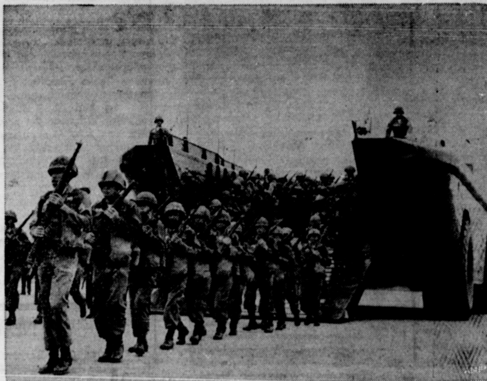
AMPHIBIOUS BARC —Troops from Fort Ord, California demonstrate troop carrying capabilities of the BARC, the Army's 60 ton amphibious resupply cargo barge. The vehicle can be used to transport heavy and bulky cargo from ships off shore across the beach to scene of operations. Both Western Gear and Peterson Builders, Inc. are contractors for the BARC.
