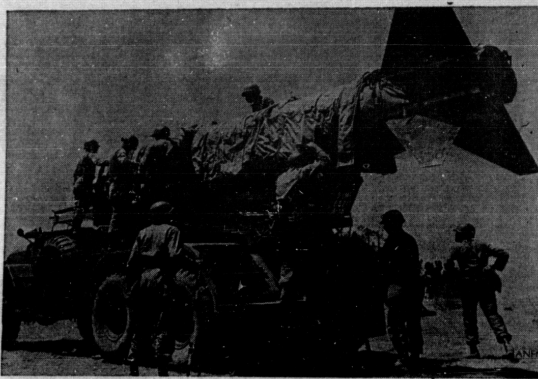
ARMY'S HONEST JOHN ROCKET with heating blanket being removed by men of the 21st Artillery (HONEST JOHN), 5th Infantry Division (Mech.), Ft. Carson, Colo. Capable of carrying both nuclear and high-explosive conventional warheads, the HONEST JOHN was developed to supplement Army's division, corps or field army artillery. With battlefield mobility comparable to that of conventional artillery, one explosive round can deliver the demolition effect of hundreds of artillery shells on the target. Douglas Aircraft Co. is prime contractor for HONEST JOHN.
