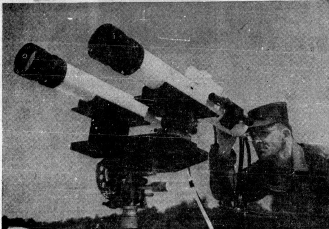
TELESCOPIC "RADAR"—LASER (Light Amplification by Standard Emission of Radiation) light is tested for radar application by this dual-telescopic device designed at the Army Signal Research and Development Lab, Ft. Monmouth, N. J. A pencil-thin beam of ruby-red light is fired at a distant object from one of the telescopic tubes and the reflection is registered in the other. The device, operated by Sp6 Eugene Medcalf of Seattle, Wash., could be a forerunner of an extremely compact device to enhance the capabilities of future defense radars.
