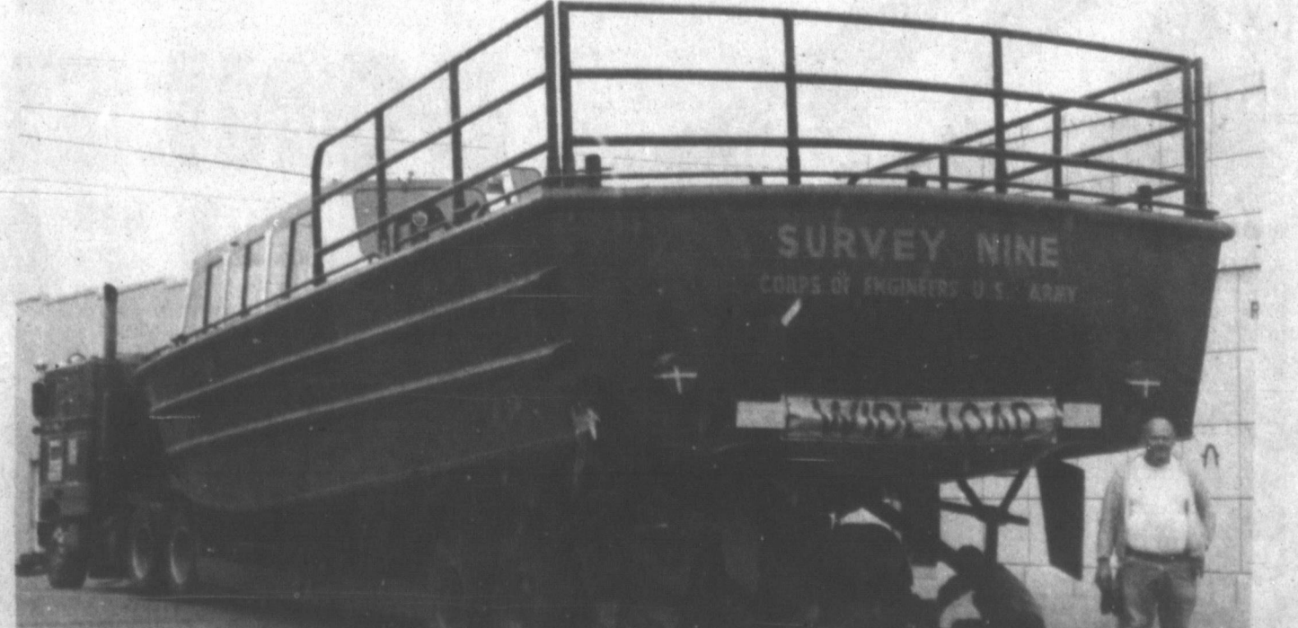
Bound for Portland, Oregon, shipyards to Vicksburg, Mississippi, this 40-foot flat-bottom boat's truck trailer blew a tire, and driver Jay Mann, pictured above, pulled into Henson's Auto Parts to make the repair. The boat, he said, will do 30 miles per hour and will be used by the Army Corps of Engineers to survey the Mississippi River. It is powered with two 450-hp diesel engines.
