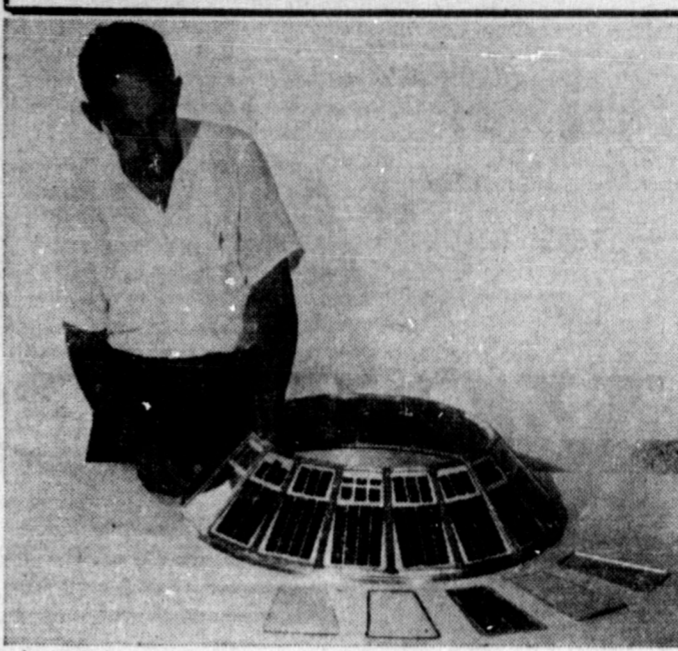
POWER FROM SOL — U. S. Army civilian space electronics engineer Andrew Herchakowski holds two rings of solar converters (sun batteries) in the approximate position they will occupy on Army-launched satellites. The rings, powering the satellite's instruments and radios with a full five watts, were developed by Herchakowski and George Hunrath of the Army's Signal Corps research and development laboratories, Fort Monmouth, N. J.
