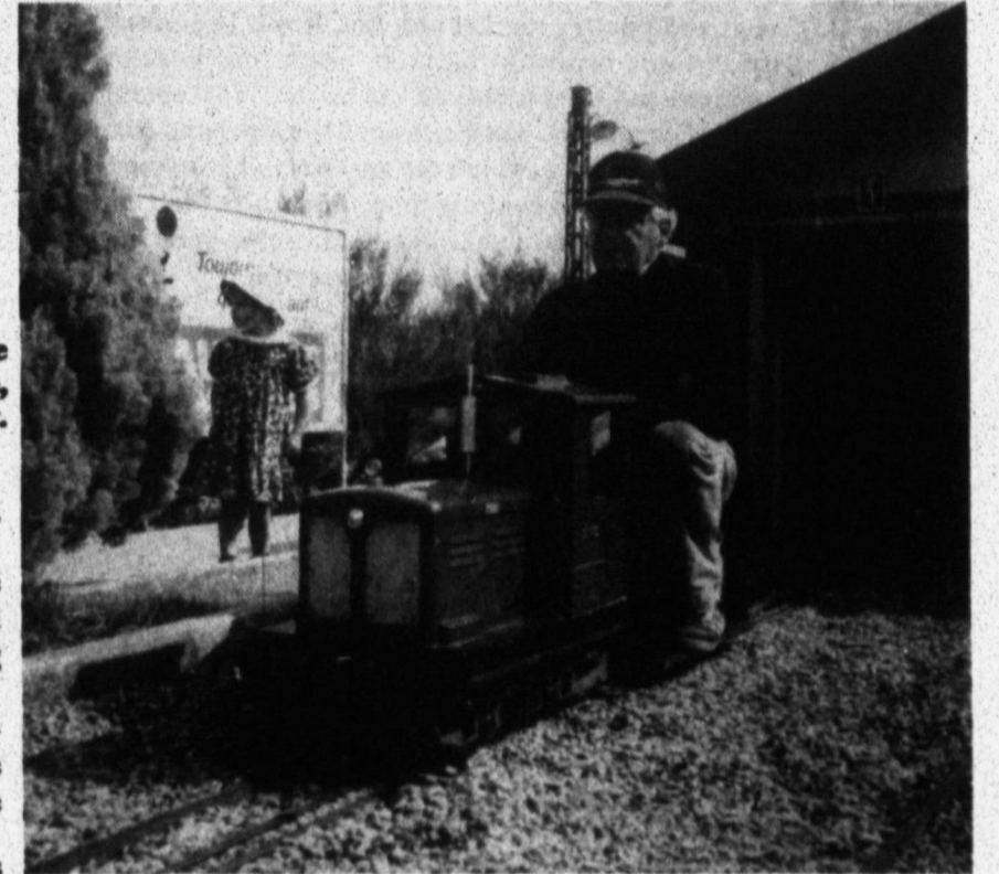
Fred Stauffer pulls out of the engine house and heads for a waiting train. His little diesel switcher is modeled after The Golden Pass, a locomotive on the Montreux-Oberland Bernois. The locomotive will pull 18 adults. It is powered by a little air-cooled gasoline engine via hydraulic drive.
