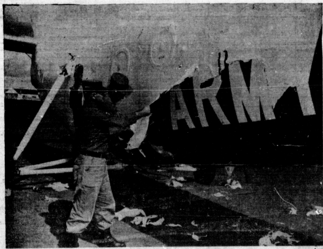
NEW ARRIVAL—Sp5 Bernard P. Murphy (St. Louis, Mo.), left, and Sp5 Wayne N. Griffith (Cuyahoga Falls, O.), members of the 545th Trans. Det., strip the protective "cocoon" off an Army H-21 SHAWNEE helicopter. The chopper, part of the equipment of the 81st Trans. Co., was sprayed with preservative to protect it from salt spray and other abrasives during its ride from California on the flight deck of a carrier. Both the 545th and 81st are attached to the 25th Inf. Div., Schofield Barracks, Hawaii. The H-21 is manufactured by Vertol Division, Boeing Airplane Co.
