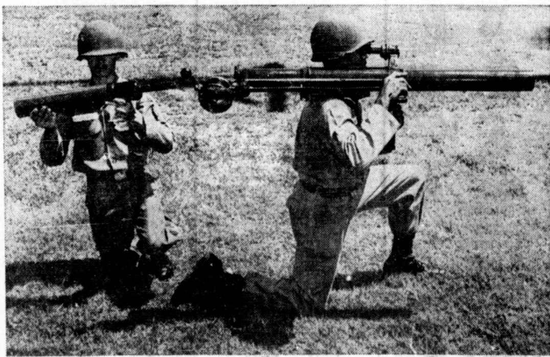
PERSONAL ARTILLERY is provided the modern U. S. Army infantryman with the development of this shoulder-fired 90 millimeter recoilless rifle—arming him with the punch of a medium-sized tank gun. Known as the MAW (Medium Assault Weapon), the 35-pound four-foot long weapon is de-
